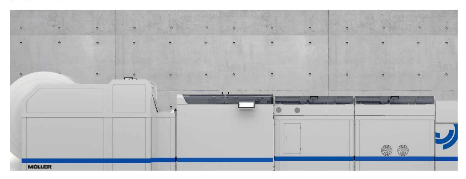
The **CONTINUOUS CHANNEL** from Müller meets a wide range of requirements in modern document processing: pinless, pinfeed, from the roll or from fan fold. It trims 60,000 A4 documents per hour with a single or double cut. Waste sheets are diverted fully automatically by means of white paper management, 2-up documents are merged and turned for flats processing without loss of performance. DL, C5 and flats applications can be processed in the same channel without changeover.
