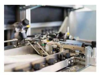
The documents are collated in the grouper according to the evaluation from the full-page reading. The 4-pocket folder has been optimized to process variable groups of up to 15 sheets. All types of fold and document lengths can be set using the AutoSet function.
