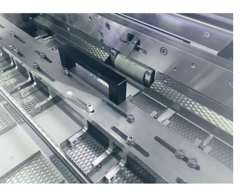
Highly stable paper path, running up to 60,000 documents in A4 per hour. Multi gains up to 4-up can be processed at a web width of 560 mm. Gross formats will be cropped 4-sided to the net format. The cutter works at the horizontal (slit and gutter cut) and vertical cuts at full speed. Waste sheets will divert by the whitepaper-management. The use of highly durable knives allows long maintenance intervals.
