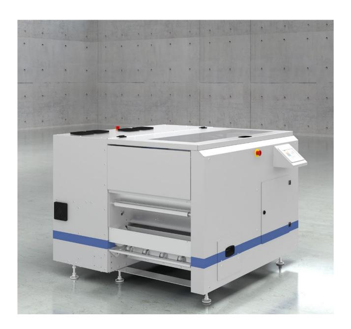
The paper web can be processed up to 150 m/min code-controlled before cutting. Horizontal and vertical perforation patterns, for example, for payment cards and coupons, filing holes or a pin strip edge strip can be applied.
