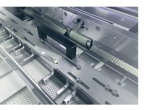
Highly stable paper path, running up to 50,000 documents in A4 per hour. Multi gains up to 2-up can be processed at a web width of 560 mm. Gross formats will be cropped 4-sided to the net format. The cutter works at the horizontal (slit and gutter cut) and vertical cuts at full speed. Waste sheets will divert by the whitepaper-management. The use of highly durable knives allows long maintenance intervals.
