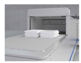
The grouped documents are accelerated and placed on the stacker separated into groups. The stacks can be deposited on the delivery belt without getting caught up in one another. It is therefore easy for the operator to remove the stacks. When the end of the stack is reached, the stacks are passed onto the next delivery belt. Through an integrated clipboard the system works also while stack exchange without interruption. The height of the stack is around 2,000 sheets at 80 g/m².
