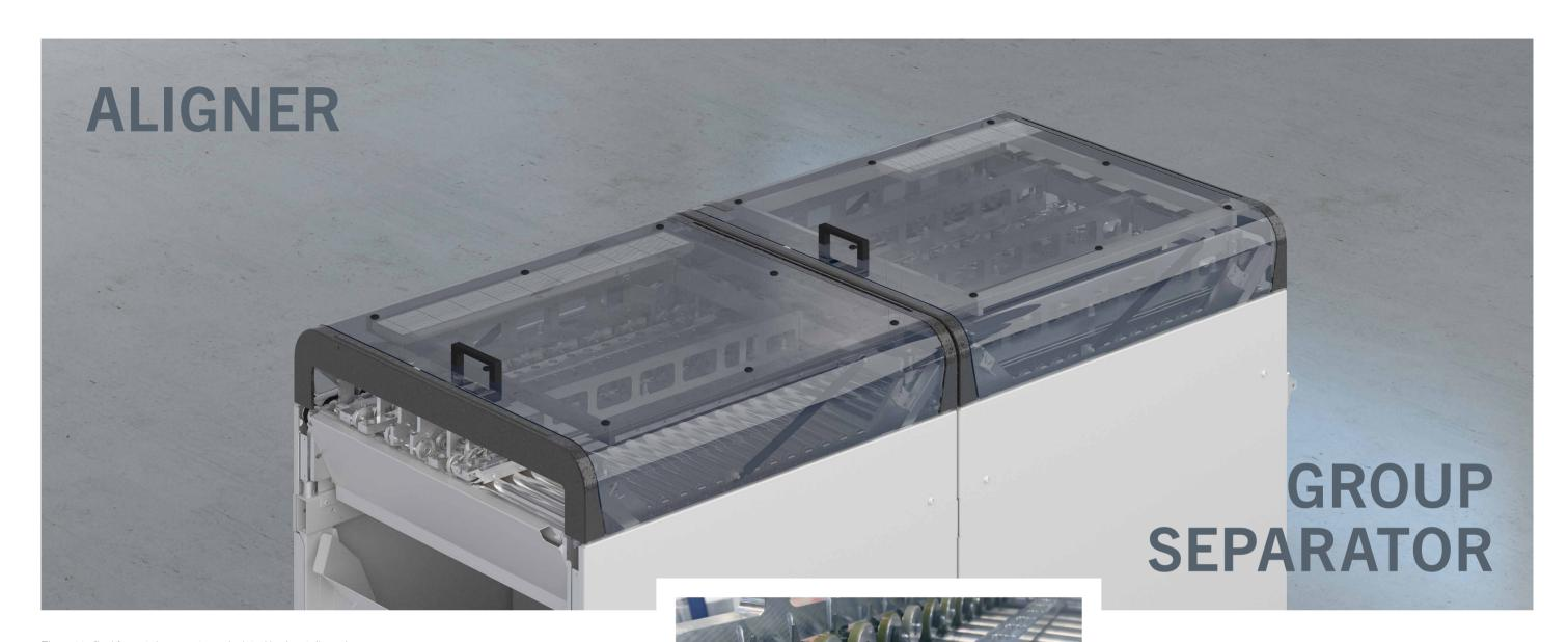
The cut to final format documents are isolated horizontally and aligned vertically. Thus, 2-up applications can be processed without longitudinal cut-outs. The productivity can be increased by over 30 percent especially with books or the American Invoice 5 ½ format, that are not printed full bleed.
