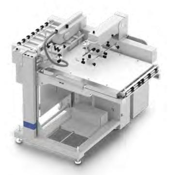
In online processing, the sheet is passed from the printer to the Müller BookTrim through the feeder. In offline processing, the feeder guides manually fed stacks to the Müller BookTrim. During this time, the printer can be used for the production of separate jobs.
